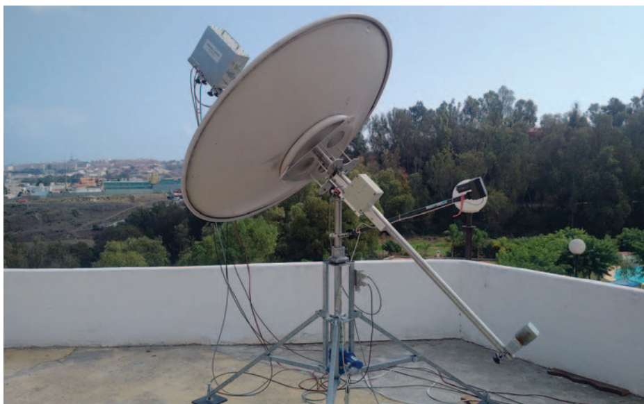
OK1DFC's 3cm EME setup in Ceuta as EA9LZ. Photo: OK1DFC.
