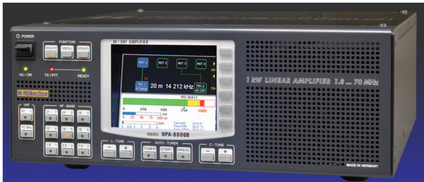
The Hilberling HPA-8000B is a linear amplifier capable of producing up to 1kW output on the 160 to 4m bands (excluding 60m).
