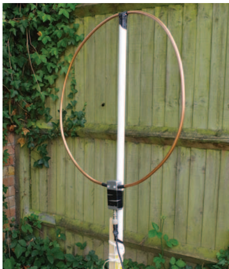
PHOTO 1: Broadband active loop antenna, useful from 400kHz to 30MHz.
