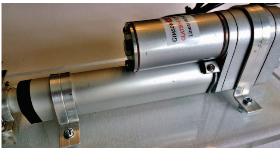
PHOTO 2: How the actuator is clamped to the Perspex base plate using homebrew straps.
